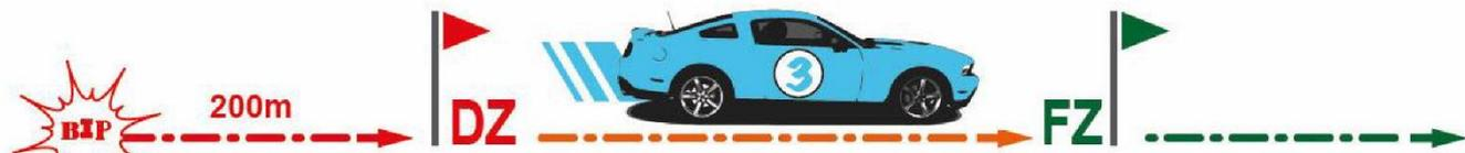
Automatic triggering of a visual and audible alarm 200m before the start of a speed zone. Continuous beep if the authorized speed is exceeded in the zone.
